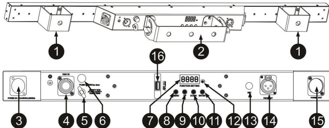
1. **SIDE BRACKETS:** with holes for mounting clamps. These can be used for linear line-ups
