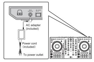
6 Press the [0] switch on the rear panel of this unit to turn this unit on.
