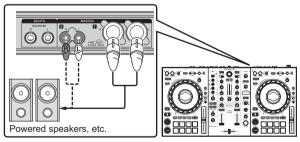
To output the sound from the [BOOTH] output terminals, connect devices such as speakers to the [BOOTH] output terminals. 3 Connect your PC/Mac to the unit via a USB cable.
