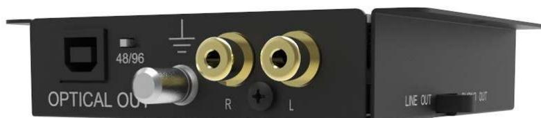
Take care to connect the left and right channels correctly. The right channel is usually marked red, the left channel black or white. The earthing wire of the tonearm lead should be connected to the earth terminal on your amplifier (if provided).
