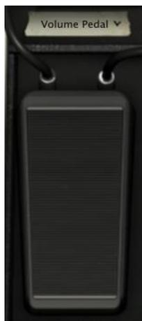
This works as a volume pedal that is assigned to MIDI CC #7. You can also click and drag on the pedal to change the volume amount.
