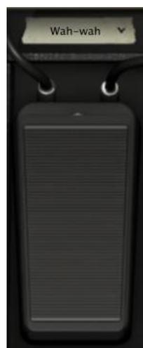
This works as a standard wah-wah pedal. It defaults to being assigned to being assigned to MIDI CC #11 Expression. You can also click and drag on the pedal to change the wah-wah frequency.
