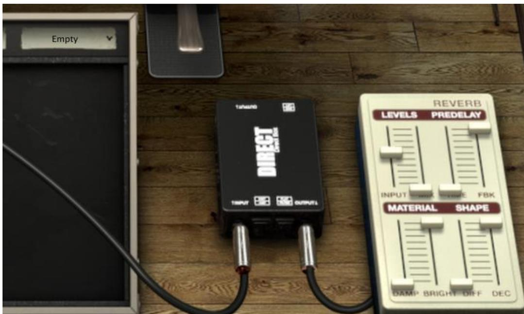
The Wurlitzer V, and the effects are connected to a direct box, that will allow you to listen the pure sound on the output. There is a reverb that follows the direct box, just as it would be in a studio.
