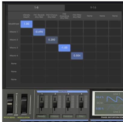
The modulation sources we’ve selected are listed on the left side (row headers) and the modulation destinations we’ve selected are listed along the top (column headers). The blue boxes show the connection and level of modulation from a source to a destination.
