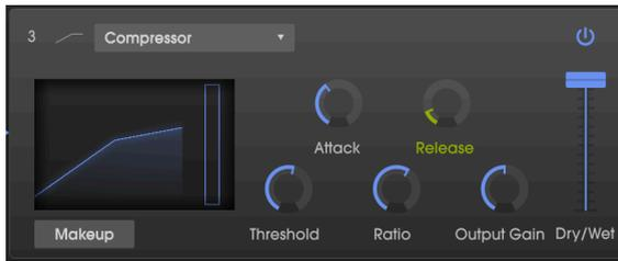
A compressor is an automatic level control. If a signal rises above a certain level (the threshold), the compressor lowers the signal output to compensate (at low Ratios) or won't let it rise at all (high Ratios, also called "limiting"). It is generally used to help maintain a consistent level of sound, though there are many other ways to use it.
