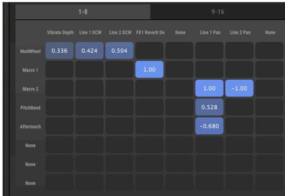
Each of the 16 mod routings allows up to 8 different sources to be routed to a single destination, or as many as 8 destinations to be modulated by a source.
