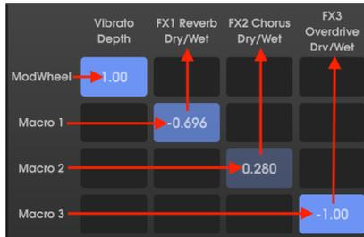
The above example maps single sources to single destinations. But you can map one source to multiple destinations, or have one destination modulated by multiple sources, like this:
