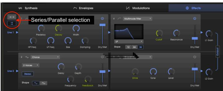
*The same effect modules as in the first illustration, but in parallel mode. Line 1 is going through a Reverb into a Multimode Filter, and Line 2 is going through a Chorus into an Overdrive. Note the addition of the Line 1 and Line 2 volume controls on the right side.*
