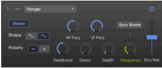
Flanging works by mixing two nearly-identical signals together, with one signal delayed by a small and gradually changing period. This produces a swept “comb filter” effect as the delayed signal adds and subtracts from the original due to phase cancellation at multiple frequencies simultaneously.
