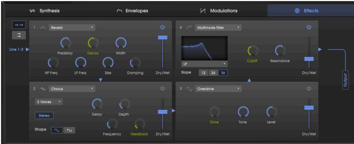
*FX page with a serial chain of four digital effects: a Reverb into a Chorus into an Overdrive into a Multimode Filter. Follow the blue arrows to trace the signal flow. The green controls are available as Mod destinations in the Mod matrix.*
