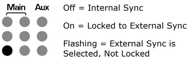
The bottom left LED in the Mode Display is the Ext Indicator. If the Ext LED is off, then the ADC1 USB is set to operate at a fixed sample rate using the internal clock source.
