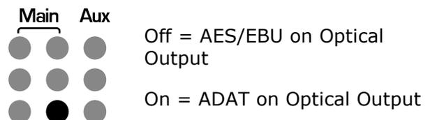
When ADAT is active, S/MUX is automatically enabled at all 2X and 4X sample rates (88.2 kHz, 96 kHz, 176.4 kHz, and 192 kHz).
