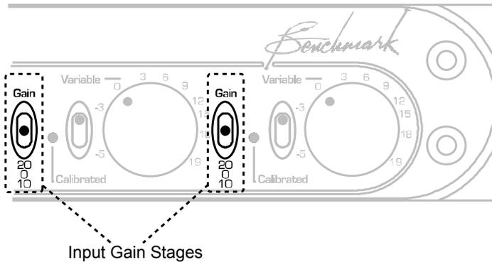
The First-Stage Gain Switches can apply analog gain (0, 10, or 20 dB) to the left and/or right channel. Both channels have their own dedicated switches. The First-Stage Gain can be used in 'Calibrated' or 'Variable' mode.
