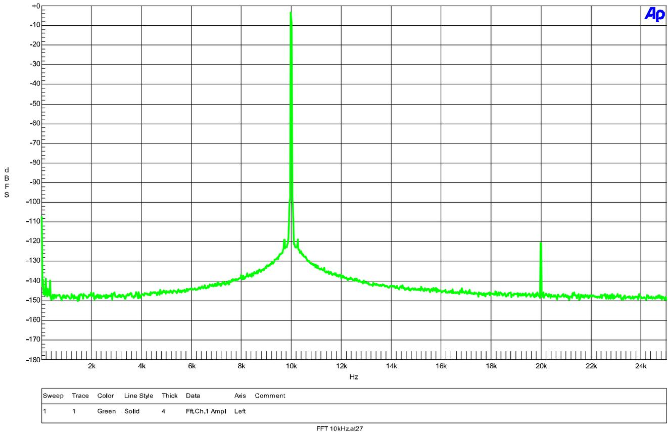
The above FFT plot shows that the ADC1 USB is free from jitter-induced sidebands. Any jitter present at the conversion sampling circuit would produce sidebands equally spaced above and below the 10 kHz test tone. The tone at 20 kHz is due to second harmonic distortion, and measures almost 120 dB below full scale. Note the near absence of spurious tones.
