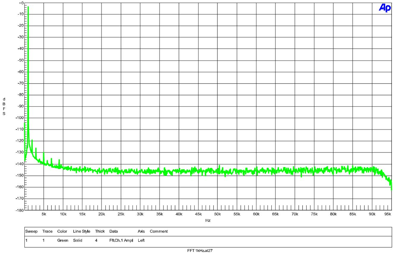
The above FFT plot shows that the ADC1 USB has very little harmonic distortion. Distortion is exceptionally low and is dominated by 2<sup>nd</sup> harmonic distortion. Note the near absence of spurious tones.
