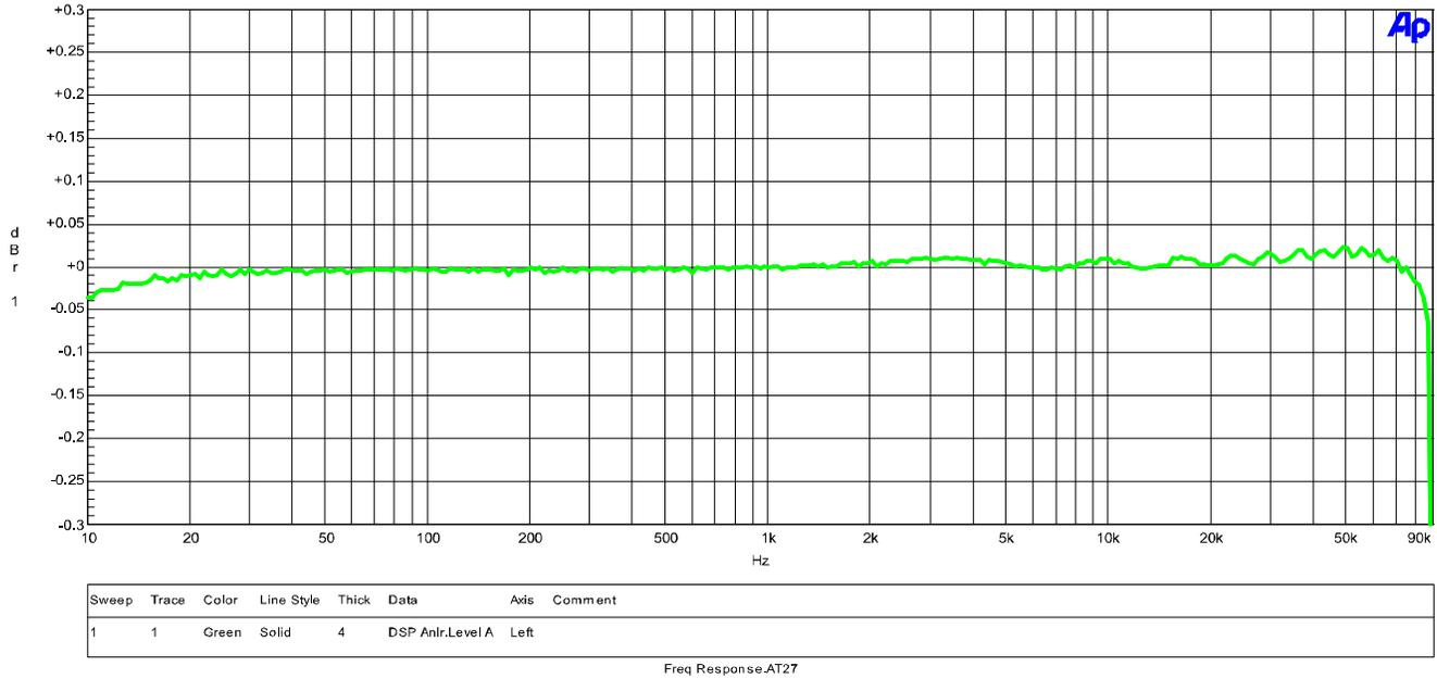
The above graphs show the frequency response of the ADC1 USB when it is operating at a 192-kHz sample rate. Note that the amplitude response is down by less than 0.05 dB at 10 Hz and 80 kHz. The bass response extends well below the 10-Hz limitation of the measurement equipment, and the high-frequency analog response extends well above the 96 kHz bandwidth of 192 kHz digital audio.
