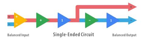
In detail: The balanced input signal will first be converted into single-ended operation by extra circuitry added to the single-ended signal path. The volume control and actual headphone amplifier are formed by a pure, single-ended circuit.
