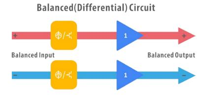
In detail: The Pro iCAN circuit is fully-balanced with completely equal circuit sections for Positive (Hot) and Negative (Cold) signal phase of each channel. The Volume control has 6-Decks, two decks each control the volume of one channel, and the other two decks are used for monitoring the volume control operation. This exceptional volume control potentiometer is custom made for iFi by ALPS Japan and has no parallel from other makers.
