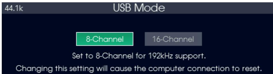
The Aurora<sup>(n)</sup>-16 USB has a unique page to itself. The LT-USB can operate in two different modes, 8-Channel and 16-Channel. In 8-Channel mode, 192kHz operation is possible, however in 16-Channel mode 96kHz is the maximum sample rate. This page allows switching between the two modes. Please note that changing the setting will reset the computer connection.
