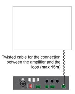
The installation consists of an electrical wire that runs through the perimeter of the room forming a loop.
