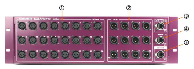
**U** Input sockets 24 balanced XLR inputs for microphone and line level sources. The preamps are built into the AR2412 rack and their Gain, Pad and 48V phantom power is remote controlled from the GLD console via the dSNAKE link. The output of the analogue preamps are converted to digital format and transported via dSNAKE to be processed and mixed at the GLD-80 mixer.
