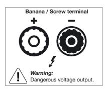
**Note:** When using stripped cables, please make sure no wire comes into contact with both polarities. Please use tinned cables to get rid of eventual short-circuit problems.
