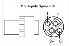
**Note**: Your speakers cables feature 2-pole Speakon® connectors can still be connected to the 4-pole outputs.
