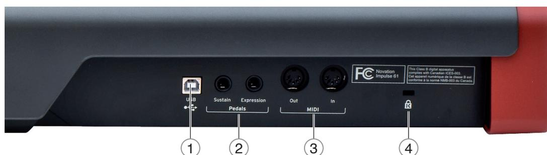
1 **USB port** – USB Type B connector compatible with USB 1.1, 2.0 or 3.0. Connect the Impulse to a USB port on your computer using the USB cable supplied. Alternatively you can connect a USB AC-to-DC adaptor here if using Impulse away from a computer.
