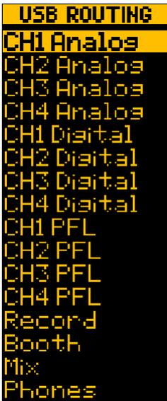
This menu selects the routing options for the upstream USB. Send 1 corresponds to USB 1-2, send 2 to USB 3-4 etc. The options are:
