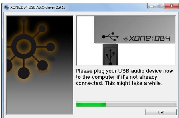
5— When prompted, connect the DB4 to the PC with the USB lead.
