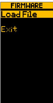
Use a good quality USB key of between 32MB and 4GB. Copy any files that you need to keep, then format the key using FAT32.
