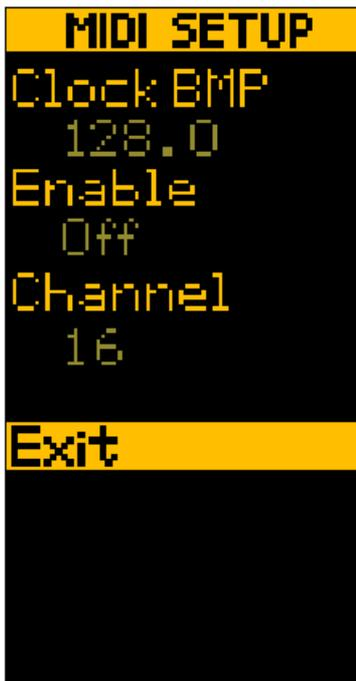
From Version 2 firmware, the Xone:DB4 has the ability to generate internal MIDI clocks which can be used to control the tempo of a connected DAW via USB.
