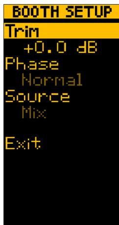
**Trim:** Sets the signal level of the Booth outputs. 0.0dB corresponds to a nominal output level of +4dBu when the main meters read 0vU. This is an ideal level to feed power amplifiers or interface with pro audio equipment. If the Booth level is too high, it can be attenuated by up to 40dB.
