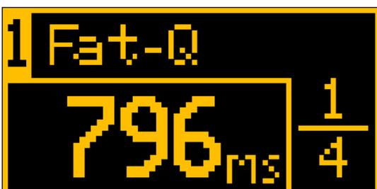
Whilst adjusting the delay time in milliseconds, the beat fraction will increase or decrease accordingly. This is represented by the fraction numbers shifting along the fraction dividing line.
