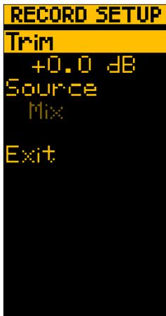
**Trim:** Sets the signal level of the analogue record outputs **and** the Digital Output. 0.0dB corresponds to a nominal output level of +4dBu when the main meters read 0VU. This is an ideal level to feed power amplifiers or interface with pro audio equipment, but is too high for most recording devices, (minidisks etc) so use this control to attenuate the output level by up to 40dB.
