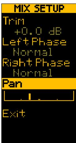
**Trim:** Sets the signal level of the Main Mix outputs. 0.0dB corresponds to a nominal output level of +4dBu when the main meters read 0vU. This is an ideal level to feed power amplifiers or interface with pro audio equipment. If the Mix level is too high, it can be attenuated by up to 40dB.
