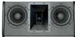
This speaker remains one of our most popular choices for speech reinforcement, for under-balcony and on-wall locations in permanent installations, and as a high-quality monitor system. Dual 8" drivers in a tuned enclosure are matched to a 1" titanium compression driver with a 100° x 100° Constant Directivity waveguide.
