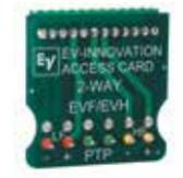
EV Innovation Access Card lets you test EVA, EVF or EVH transducers and protection circuitry without disassembling the cabinet.
