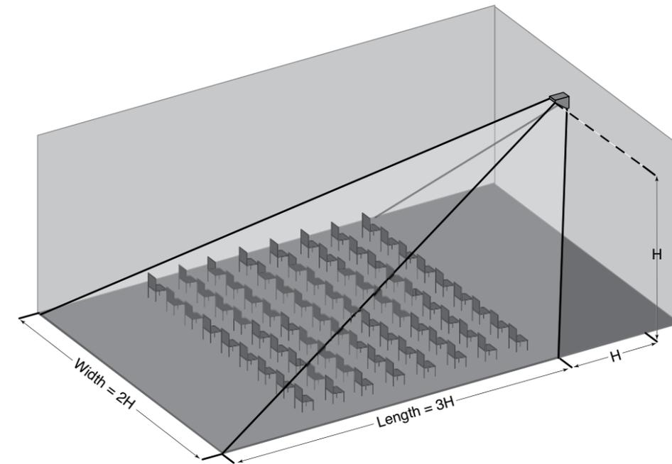
EVI provides a simple, economical solution for permanent installations requiring even coverage over a fixed rectangular area. In a typical room, the distance from a front-mounted loudspeaker to the last row is two or more times the distance to the front row, resulting in a substantial front-to-back difference in level and
