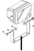
Note: The thread diameter can be reduced with a standard 5/8" screw adapter for different mic stands.
