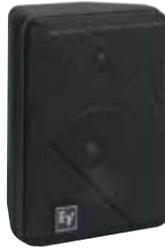
Delivering high performance in an ultra-compact package, the S-40 is ideal for both distributed and near-field applications requiring high-quality sound. The two-way short-throw system is housed in an optimally vented, high-impact polystyrene enclosure that is suited for installation both indoors and out. Lows are handled by a 5.25" direct-radiating woofer with a polypropylene cone, while the high-frequency section is a
