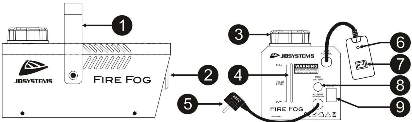
1. **HANGING BRACKET:** hanging bracket with two knobs on both sides to fasten the unit + mounting holes to fix a mounting hook.
