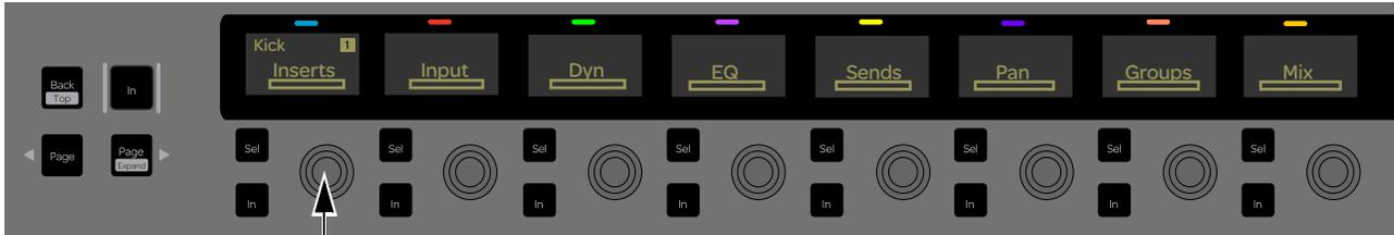
The Channel Control displays now show the available Inserts slots. If no plug-in is inserted in a slot, the slot letter appears in lower-case (a, b, c, and so on) in the corresponding display. If a plug-in is inserted in a slot, the name of the plug-in is shown in the corresponding display. Plug-in names are abbreviated as necessary.
