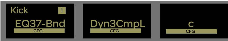
*Insert slots a–c (left-to-right) in Config mode in Channel Control*
