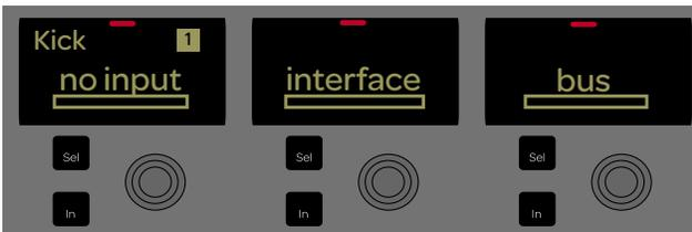
Channel Controls displays showing available input types
