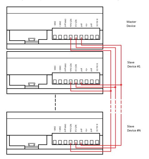
Interfaces configured as slave will strictly follow the clock, triggers and information providing by the master interface. Only one master interface at a time is possible.
