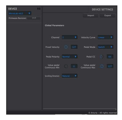
Editing MicroLab mk3 parameters in MIDI Control Center is simple. Various editable parameters are shown on the right side, and all changes are sent automatically to MicroLab mk3.
