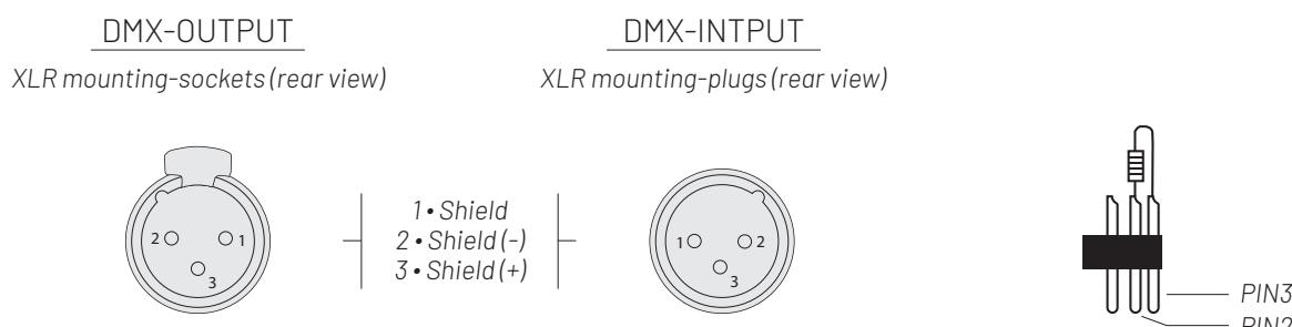
When using standard DMX512 control signal, the last device's output interface must be connected to a DMX plug. This plug is putting a 120 ohm resistance between "canon" plug's 2 pin and 3 pin. Showing as below pic. Sticking this plug into the last device's signal output interface, it will avoid the interference during the process of signal transmission.
