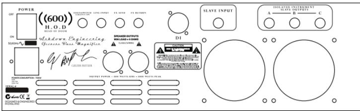
**SLAVE INPUT** - There is a slave input on the rear of the head this has been designed to be fed by the transformer isolated outputs if running multiple heads from one input source...
