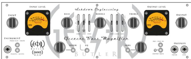
**INPUT** – There is a single instrument input provided linked to a PASSIVE/ACTIVE selector switch. The Passive input (switch out) is high sensitivity and also high impedance to suit the output from PASSIVE basses. The Active input (switch in) is low sensitivity and lower impedance to suit the output from ACTIVE basses.
