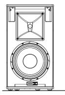
Horn in its original position when the speaker is used vertically.
