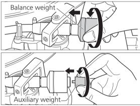
Attach the included auxiliary weight to the rear of the tone arm according to the weight of your cartridge.
