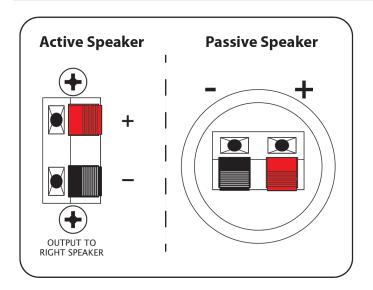
**Bare-wire connectors.** This connection is used to send power and signal to the passive speaker. Be sure to connect the positive and negative connections on your active speaker to the positive and negative connections, respectively, on the passive speaker (i.e. connect positive to positive and negative to negative).
