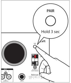
Your Eris E5 BT can be paired with any Bluetooth device for audio playback. To pair your speakers, first press and hold the pair button on the rear of the active Eris speaker for three seconds.
