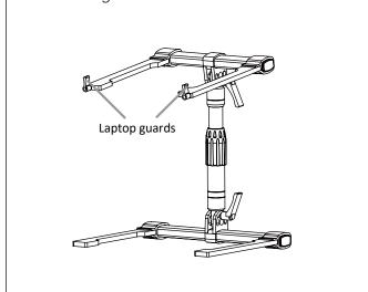
4. The stand can be set in Z position by adjusting the angle of the tray and legs, and turning the neck 180°.
