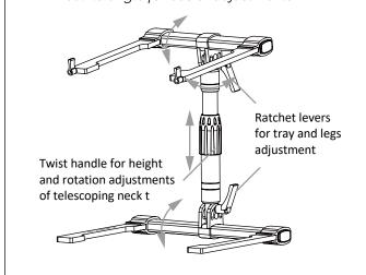
3. Unfold the laptop guards to keep laptop in place. Note: Be sure to fold the guards before folding and stowing the stand for storage or travel.
