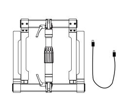
2. Unfold the stand by loosening the two ratchet levers for the tray and legs. Find your desired position and tighten the levers. Note: Pull the lever towards you to set its angle for easier adjustments.
