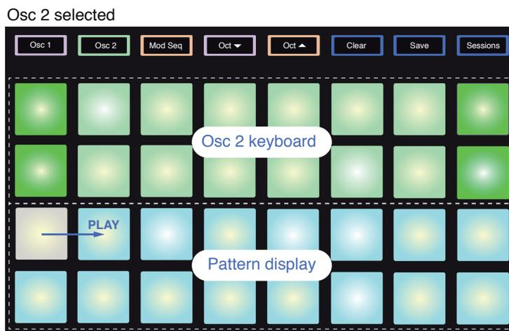
The Osc 2 level control in the Mixer section [24] must be turned up and Paraphonic mode 2 selected (by pressing **Shift + Scales**) in order for Oscillator 2's notes to be audible. Note that the **Scales** button is illuminated bright white when Mode 2 is active.
