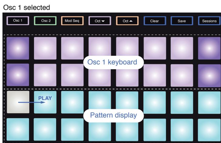
In order to hear the notes from Oscillator 1, ensure that the **Osc 1** level control in the Mixer section [23] is turned up.
