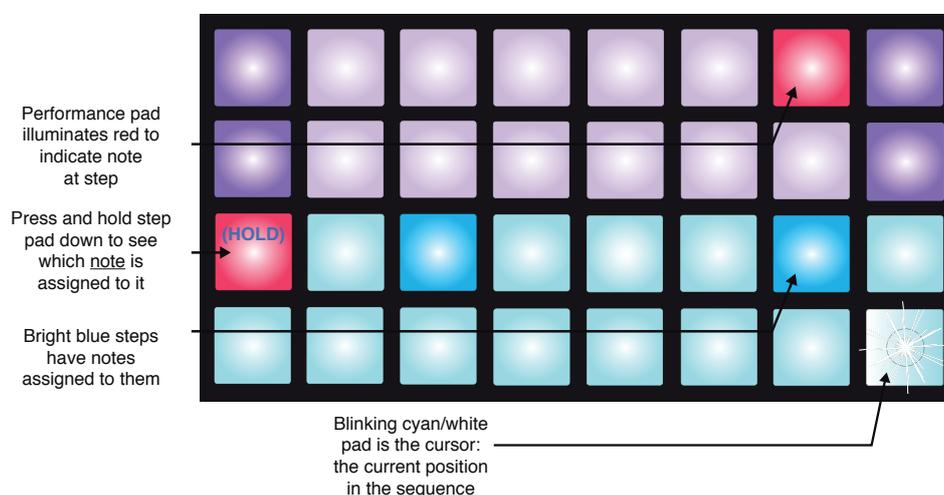
If a bright blue step pad (i.e., one corresponding to a synth note) is pressed and held, it illuminates red, the note at that step will sound, and the performance pad corresponding to the note will also illuminate red. The pad stays red and the note sounds for as long as the step pad is held down.
