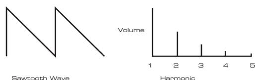
These are rich in harmonics, and contain both even and odd harmonics of the fundamental frequency. The volume of each is inversely proportional to its position in the harmonic series.
