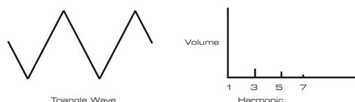
These contain only odd harmonics. The volume of each decreases as the square of its position in the harmonic series. For example, the 5th harmonic has a volume  $1/25$ th of the volume of the fundamental.
