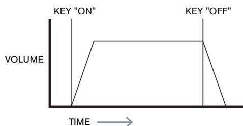
In an analogue synthesiser, changes to a sound's character which occur over the duration of a note are controlled by a section called an Envelope Generator. One (**Amp Env**) is always related to the Amplifier, which controls the note's amplitude – i.e., the volume of the sound - when the note is played. Each envelope generator has four main parameters, which determine the shape of the envelope; these are often referred to as the ADSR parameters.
