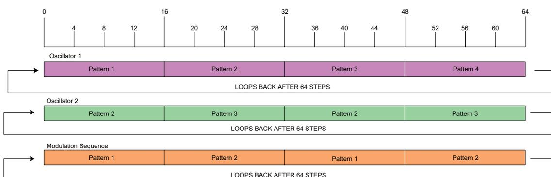
Every time you press **Play**, the Pattern restarts from the beginning of the first Pattern in the chain. You can restart the Pattern from the point at which the sequencer was stopped by pressing **Shift** and **Play** together.
