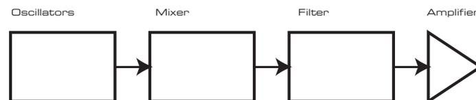
Additional synthesiser sections - **LFOs** and **Envelopes** - provide further ways of altering the pitch, tone and volume of a sound by interacting with the **Oscillators**, **Filter** and **Amplifier**,
