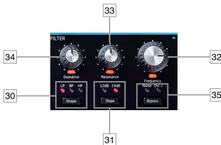
The sum created in the mixer from the various signal sources is fed to the Filter Section. Circuit Mono Station's filter section is both simple and traditional, and can be configured with only a small number of single-function controls.
