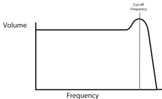
In addition to the traditional low-pass filter type, there are also high-pass and band-pass types. On Circuit Mono Station, the Filter type is selected with the **Shape** switch [30](#).
