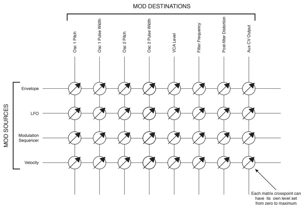
The Modulation Matrix may be visualised as a system for connecting controlling sources to a specific area of the synth. The matrix has four sources and eight destinations and thus has 32 crosspoints. The matrix is *variable*.
