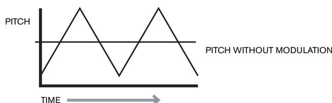
Alternatively, if the same LFO signal were to modulate the Filter cut-off frequency instead of the Oscillator pitch, a familiar wobbling effect known as ‘wah-wah’ would be the result.
