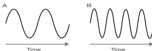
If the number of peaks in the two waveforms (vibrations) are counted, it will be seen that there are exactly twice as many peaks in Wave B as in Wave A. (Wave B is actually an octave higher in pitch than Wave A.) It is the number of vibrations in a given period that determines the pitch of a sound. This is the reason that pitch is sometimes referred to as frequency. It is the number of waveform peaks counted during a given period of time which defines the pitch, or frequency.
