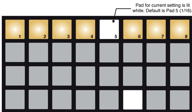
Only the top row of pads are used: one pad will be illuminated white, indicating the currently selected Swing Sync Rate, according to the table below:
