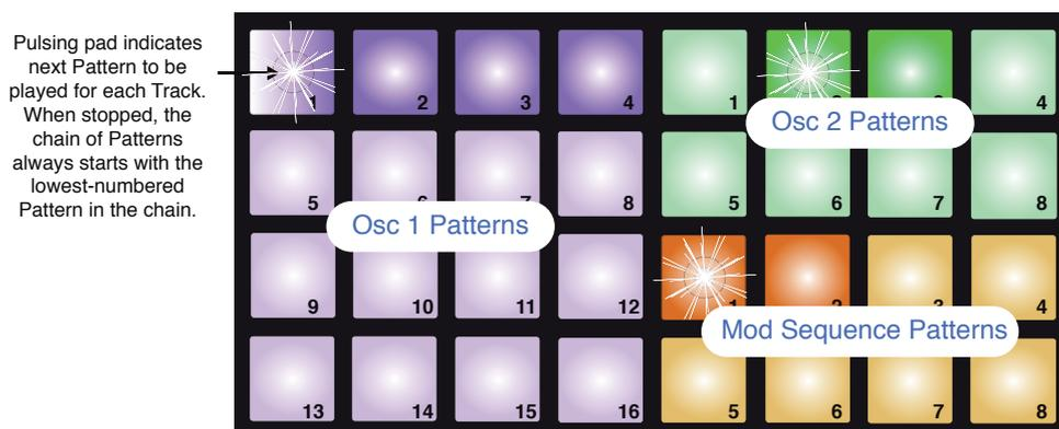
The Pattern View example above shows a possible arrangement of Patterns for a 4-pattern (64-step) sequence. We are using four Osc 1 Patterns (Memories 1 to 4), two Osc 2 Patterns (Memories 2 and 3) and two Modulation Sequence Patterns (Memories 1 and 2).
