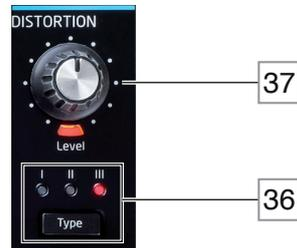
The **Type** button [36](#) selects one of three analogue distortion types, simply referred to as **I**, **II** and **III**:
