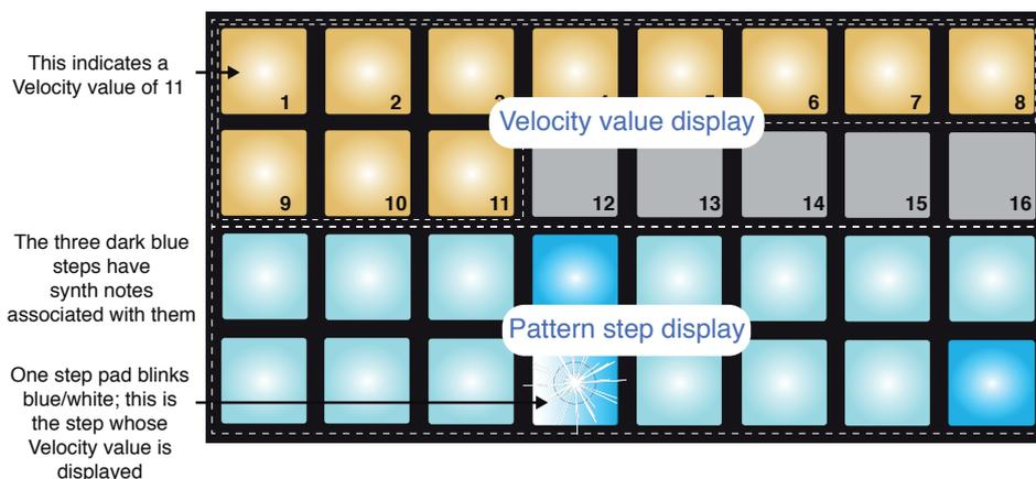
In **Velocity View**, the two lower rows of the grid represent the pattern steps. In the 16-step example shown above, Steps 4, 12 and 16 are brightly lit, indicating that these steps have notes associated with them. One pad in the Pattern step display will flash alternate white/blue: this is the step whose Velocity value is being displayed.
