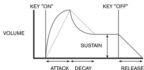
The ADSR envelope can be most easily visualised by considering the amplitude (volume) of a note over time. The envelope describing the “lifetime” of a note can be split into four distinct phases:
