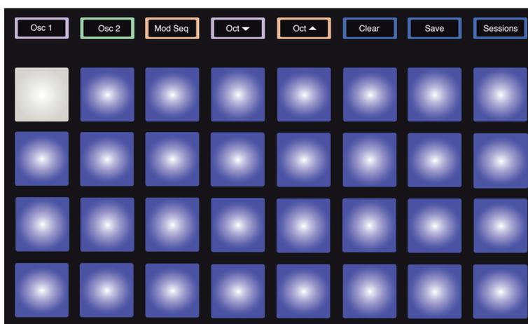
The two pages are selected with the **Oct ▼** and **Oct ▲** buttons [12](#). In Page 1, **Oct ▼** is illuminated bright white and **Oct ▲** dim white. Pressing **Oct ▲** will open **Patch View Page 2**.
