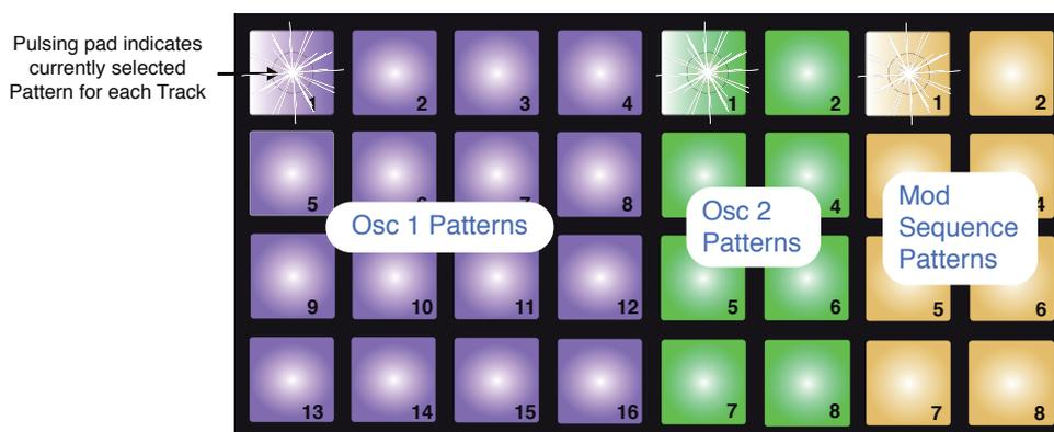
The grid is vertically divided into three areas: the first four columns of pads represent the sixteen memories for Oscillator 1 Patterns, the remaining four are divided between Oscillator 2 Patterns and Modulation Sequence Patterns. Each of the Pattern memories can contain a 16-step pattern.
