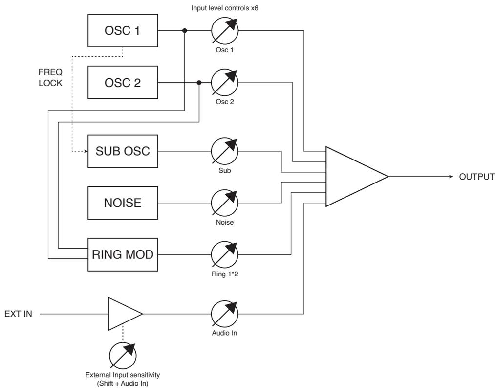
The outputs of the various sound sources can be mixed together in various proportions to produce the overall synth sound, using what is essentially a simple 6-into-1 mono mixer.
