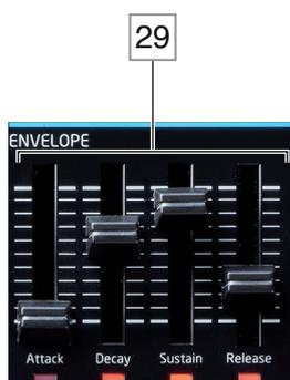
Circuit Mono Station has a dedicated slider control 29 for each ADSR parameter:
