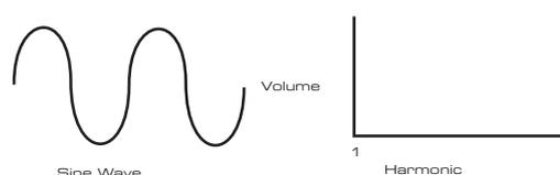
These possess just one harmonic. A sine waveform produces the “purest” sound because it only has this single pitch (frequency).
