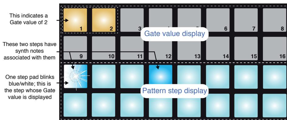
In **Gate View**, the two lower rows of the grid represent the pattern steps. In the 16-step example shown above, Steps 1 and 4 are brightly lit, indicating that these steps have notes associated with them. One pad in the Pattern step display will flash alternate white/blue: this is the step whose Gate value is being displayed.
