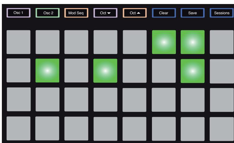
**Osc 1** and **Osc 2** are lit; selecting each of these generates a pattern of illuminated pads; the pattern represents the version numbers of the firmware elements in binary form. You may need to describe these patterns to Novation’s Technical Support Team in the event of a problem.
