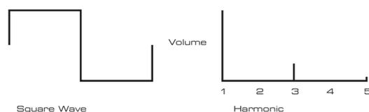
These contain only odd harmonics, which are at the same volume as the odd harmonics in a sawtooth wave.
