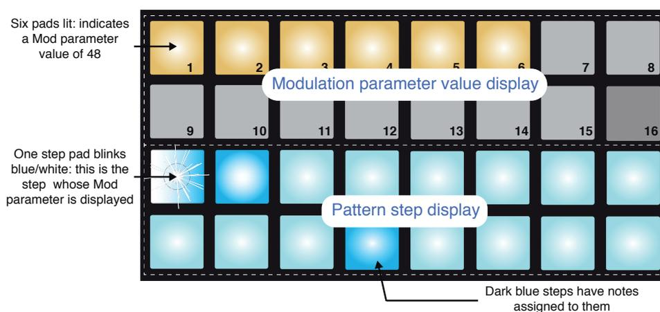
Although the value of the Modulation parameter is stored internally at 8-bit resolution (0 to 127), the restriction of 16 pads means it may only be assigned in multiples of 8, as per the table below:
