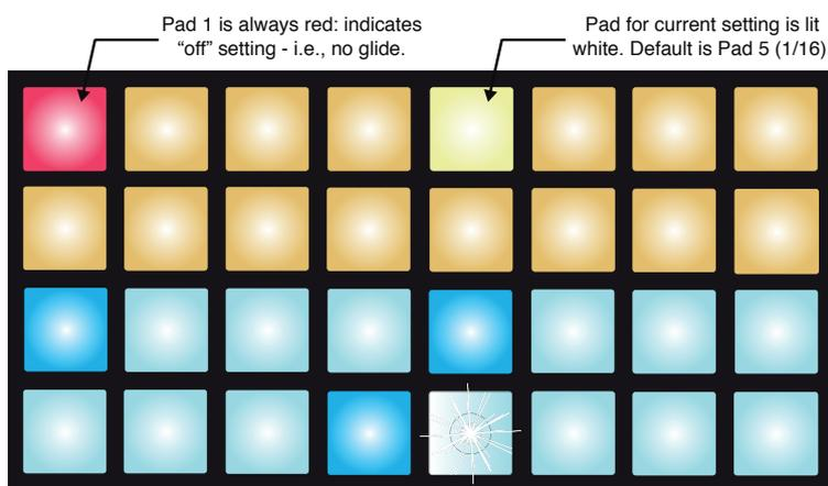
The lower two rows in Glide View show the Pattern steps, as in other Views. The upper two rows allow the Glide Time to be set for each step, to one of 16 values between 0 and 127, according to the following table:
