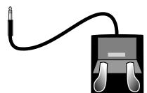
The SW1 (SUSTAIN) and SW2 jacks can be connected to dual switch pedals (2 pedals per jack), allowing up to four switch pedals to be used. Compatible pedals should use a single 1/4 inch tip-ring-sleeve plug. (Two single switch pedals can also be plugged into one jack by using a 1/4 inch stereo (male) to dual mono (female) splitter cable, aka TRS to dual TSF).
