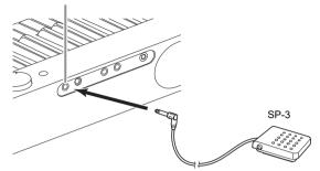
This pedal functions as a damper pedal under initial Digital Piano default settings. To change it to a different function (soft, sostenuto, etc.), see "Changing Pedal Functions" (page EN-44).
