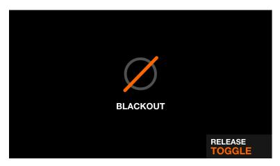
The Blackout flash effect shuts off all beams by setting dimmers to 0%, shutters closed, and color mixing channels to 0%. The effect is released according to the set release mode.
