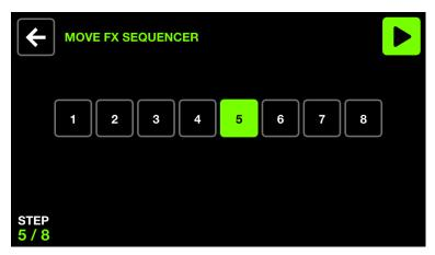
The Move Fx sequencer allows for one of four different positions to be chosen per group and recalled across eight steps. Each position will be played sequentially according to the FX speed.
