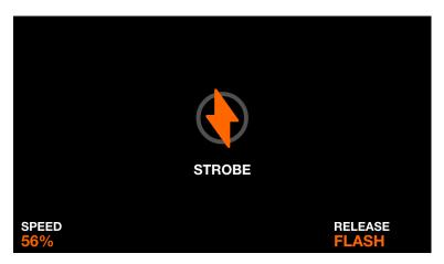
The Strobe flash effect tells all lights to strobe by triggering the fixtures strobe feature. If the fixture doesn't have a built in strobe feature, a virtual strobe will be created by flashing the RGB or dimmer channels. The effect is released according to the set release mode.
