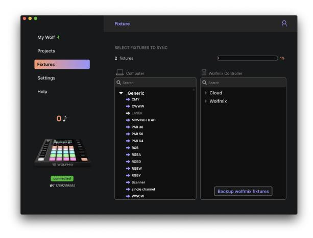
Fixtures on the computer and in the cloud are displayed on the left and fixtures in the Wolfmix controller are displayed on the right.
