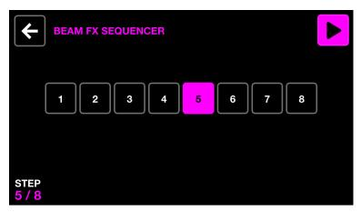
The Beam Fx sequencer allows for eight different beam selections to be chosen. When a beam selection is made, the selected beams will be opened. Each beam selection will be played sequentially according to the FX speed.
