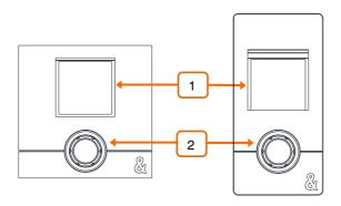
LCD Display – Colour display providing information on the selected channel or output mix. It can also display a Source or Scene list when the rotary is pressed if such function is assigned to the IP1.
