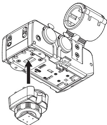
4. Use the 2 screws that were removed to affix the accessory shoe adapter.
