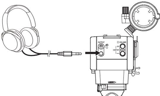
Set the OUTPUT switch (14) to  $\Omega$  and monitor the sound.
