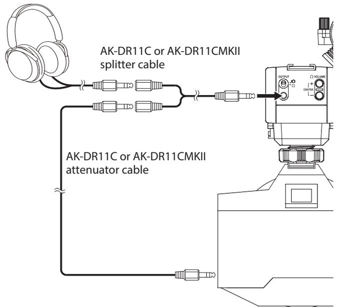
A splitter cable is necessary to monitor analog audio with a CA-XLR2d-AN.
