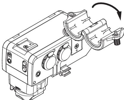
2. Place the mic in the holder, and close the holder while keeping the mic in place. Then, tighten the screw securely.
