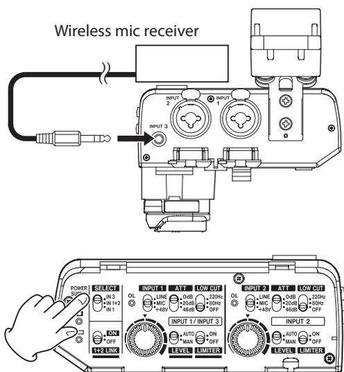
When connecting a stereo laval mic, for example, connect it to the INPUT 3 jack (21), and set the SELECT switch (2) to "IN 3".
