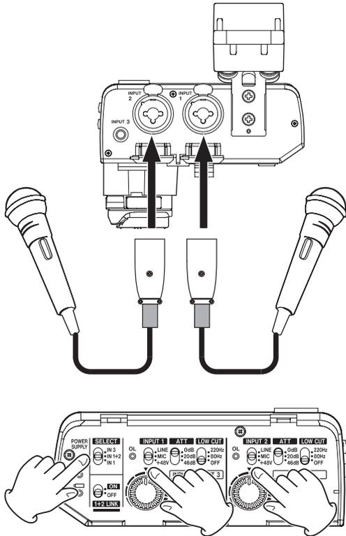
When connecting a mic to the INPUT 2 jack (20) set the SELECT switch (2) to "IN 1+2" and set the INPUT 2 switch (7) according to the type of mic connected.
