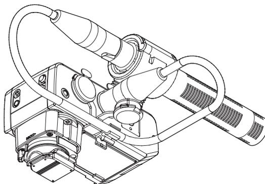
4. Set the SELECT switch (2) to "IN 1" and set the INPUT 1 switch (4) to "MIC" or "+48V".
