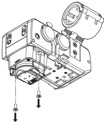
2. Remove the accessory shoe attachment adapter from the unit.
