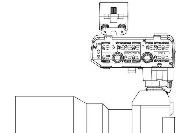
3. Using the lock lever (28) or the tightening dial (29), attach this unit to the connected device securely.
