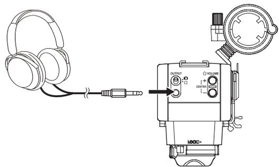
To monitor analog audio signals, set the OUTPUT switch (14) to Ω, and connect headphones or an earphone, for example, to the OUTPUT jack (15). Then use the Ω VOLUME +/- buttons (16) to adjust the volume.
