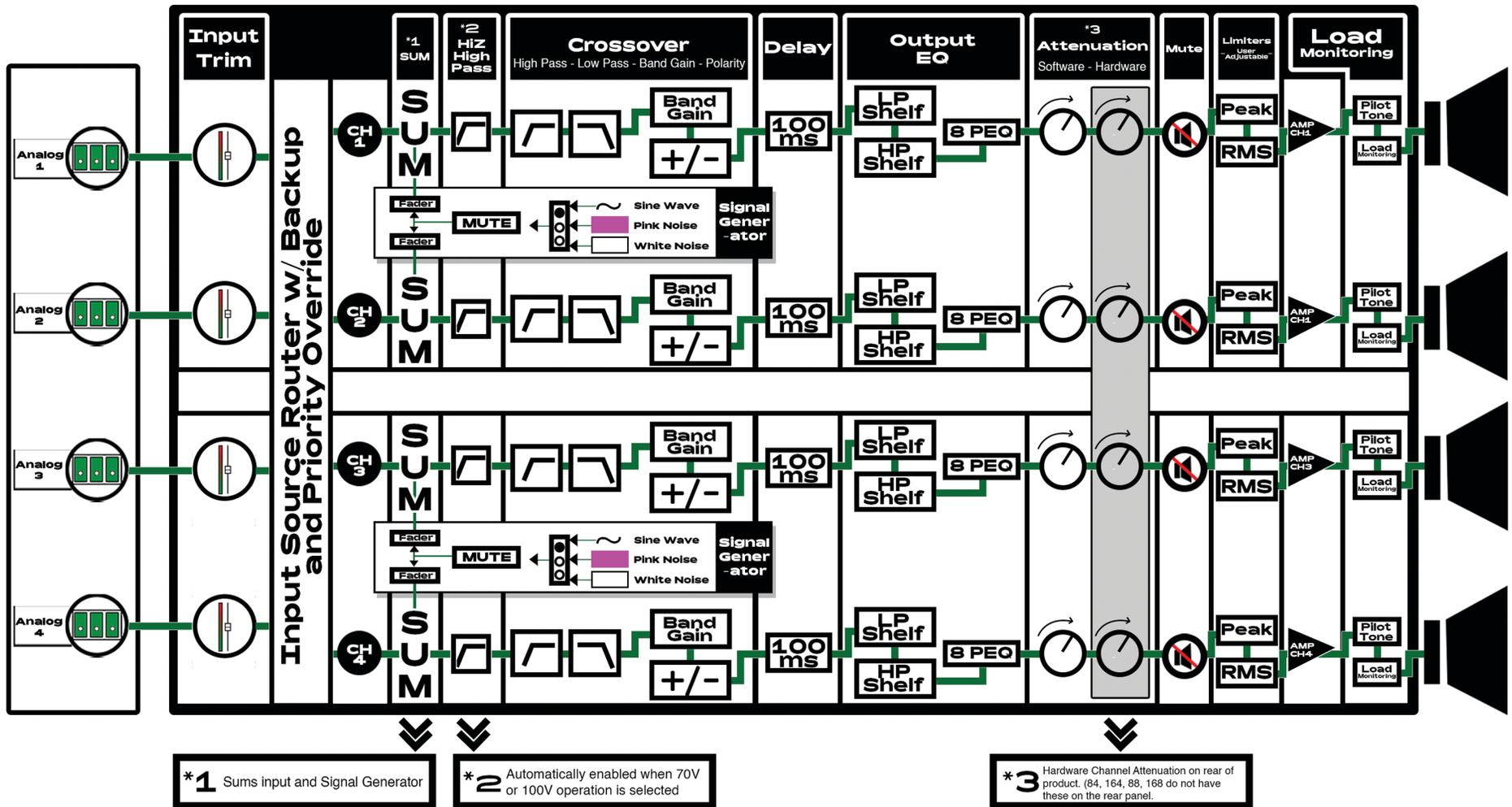
**Analog Inputs:** Balanced analog inputs with 34dB and 26dB selectable input sensitivity modes. In 34dB mode, the input sensitivity is 1.4 VRMS and allows you to achieve full output in LowZ and 70V modes. In 26dB mode, the input sensitivity is 2.0 VRMS and allows you to achieve full output in 100V mode. These modes are selectable in the input mode of the WebUI.
