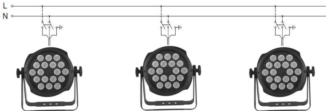
The device must be connected to a power supply system with a proper earth system. Moreover, it is recommended to protect power supply lines of the products from indirect contact and / or shorting to earth by using appropriately sized anti electrical shock switch. The electrical connection must be carried out by a qualified electrician. Ensure that the mains frequency and voltage correspond to those for which the device is designed, as shown in the electrical data label.
