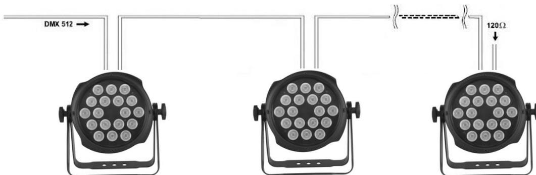
Use a cable conforming to specifications EIA RS-485: pole twisted, shielded, 120Ohm characteristic impedance and low capacity (SAGITTERSG DMX3 – SG DMX5). Do not use microphone cable or other cable with different characteristics than those specified. Terminations must be made with male / female XLR 3-pin connectors. You must enter on the last device a terminal plug with a 120Ohm resistance (min1 / 4 W) between terminals 2 and 3.
