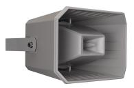
The MPLT62-G is two-way long throw horn 100 volt high quality music projector. It has 62 watts rated power handling RMS at 100 volt and has transformer taps at 62 - 32 - 16 - 8 watts. Its long throw output performance brings quality sound over long distances and in wide areas with both music and speech. The two-way characteristic makes your music still sound natural where the horn shape housing makes sure you cover a big distance.
