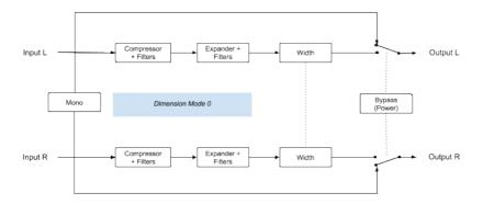
So, when Mode O is activated, the audio signal follows this path. The first stage is a Compressor + Filters. The filters act like a soft shelf-like double band EQ, which adds emphasis to the lows and attenuates the highs. This is followed by a compressor which considerably narrows the dynamics of the audio.
