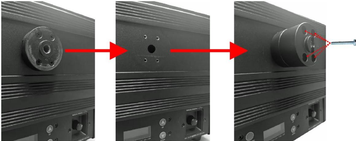
5. Instead fix the new aluminum cylinder from the BT-THEATRE YOKE and the nylon cylinder from the ADAPTER-2 set on both sides of the projector. To do this, use the 8 new M4-bolts included with ADAPTER-2 set
