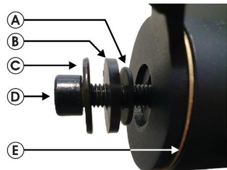
**Important remark:** don't forget the copper washer / ring (E) otherwise the tilt mechanism will not work well!
