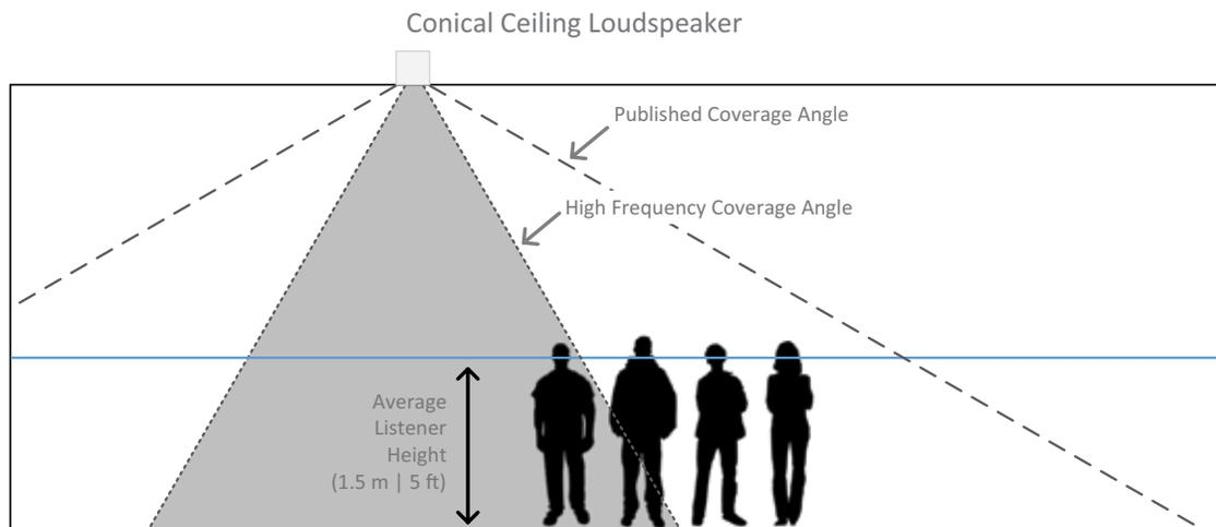
**Figure 1.** Comparison between the published and typical high frequency coverage angles for an in-ceiling conical dispersion loudspeaker. Note that the shaded section represents the area where a balanced frequency response will be delivered.
