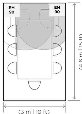
**Figure 13.** In smaller conference rooms a single EM180 can be used above the screen location, or two EM90s in the corners can provide both speech and program material reinforcement.
