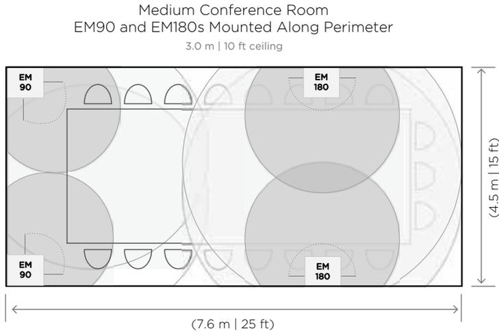
**Figure 15.** In medium-sized conference rooms two EM90s can be mounted in the front of the room for stereo playback and conferencing, while additional EM180s can be installed along the side walls for conferencing reinforcement.
