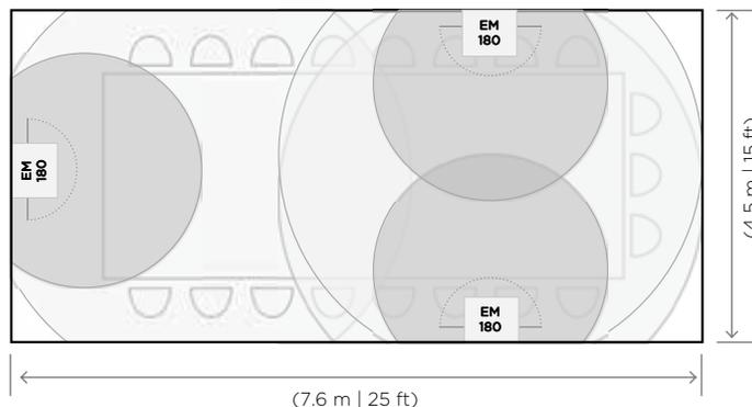
**Figure 14.** In medium sized conference rooms a single EM180 is used above the screen location, and additional EM180s along the edges provide reinforcement for audio and video conferencing.
