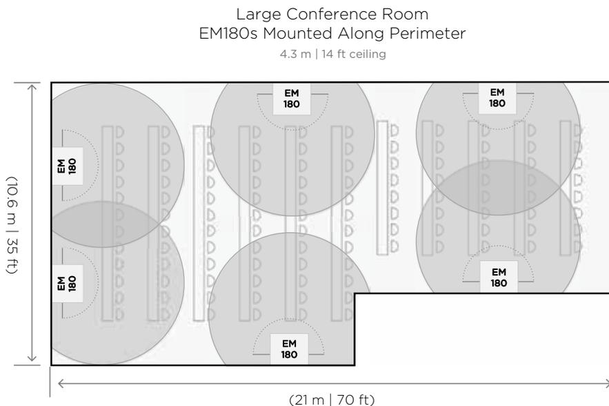
**Figure 16.** A large conference room with two EM180s mounted near the video screen location, and additional units spaced along room sides using the recommended loudspeaker spacing for the room's ceiling height.
