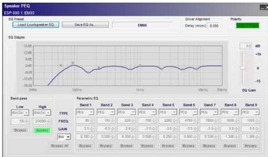
**EdgeMax EM180 loudspeaker EQ** – Use when the system contains only EM180 loudspeakers.
