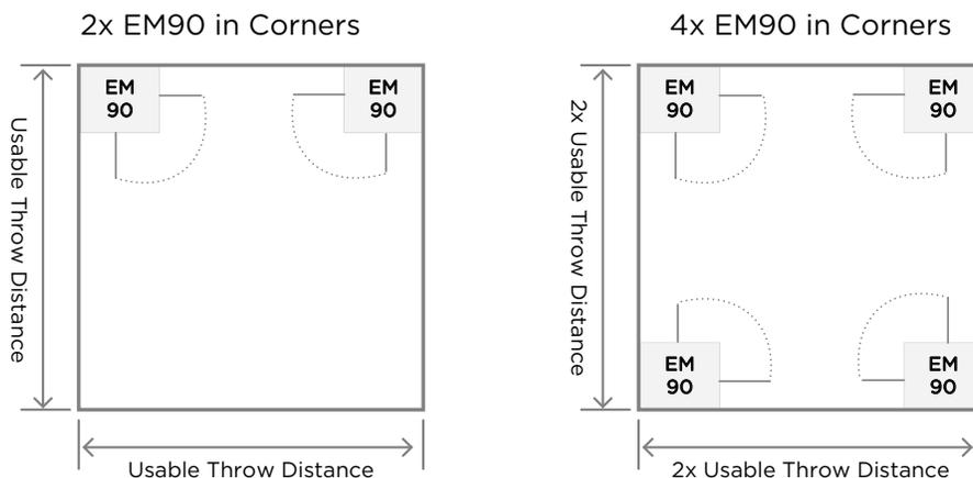
**NOTE:** For designs where bass is a primary consideration, square rooms with 4x EM90s will deliver more bass than 4x EM180s, due to the additional wall-boundary loading provided by the corner mounting.
