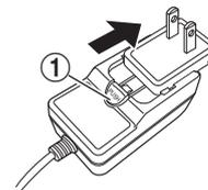
2. Once the AC adapter plug has been slid out as far as possible, lift it up in the direction of the arrow to remove.
