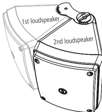
Mount the cluster to the "U" bracket by tightening other two round knobs or bolts to fix the first loudspeaker, and the two linking supports (with the second loudspeaker). Pay attention to the cluster horizontal aiming.
