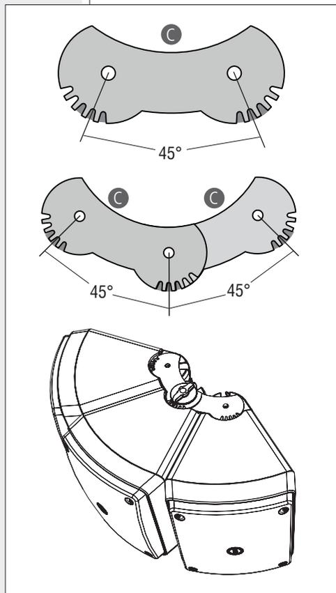
Make the cluster by putting the three loudspeakers together and fix the central one (and the four linking supports) by tightening two round knobs / bolts (up and down).
