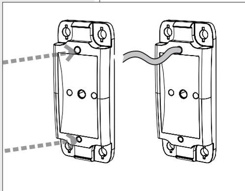
Put the "U" **B** bracket on the mounting accessory **D** and choose the right vertical\* aiming angle ( $\pm 30^\circ$ ; each hole is a  $7.5^\circ$  step), then fix it by tightening the bolt **F** through the dedicated plastic plate **E** and washer **G** and **H**.
