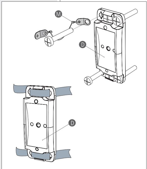
To get a weatherproof electrical connections and reduce the visible / external part of the loudspeaker cable (1 m long), this can pass through the "U" bracket, the mounting accessory hole (to be opened by pressing the plastic in one of the two available points) and its back seat, then inserted into the wall niche\* (behind the mounting accessory) that houses electrical connections.
