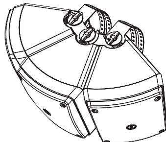
Now the cluster is ready to be fixed to the two wall-mounted accessories by tightening the two bolts.
