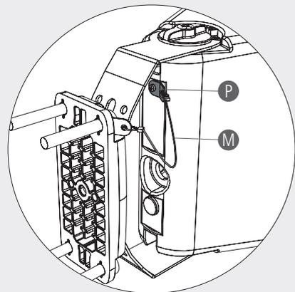
Use a screw **P** to fix the safety steel cable **M** as shown in this example.
