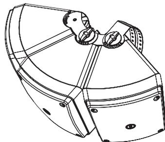
Then add the other "U" bracket (the left one in this example) under the linking support and tighten the relevant two (up and down) round knobs / bolts.
