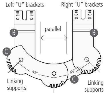
First mount the "U" bracket (the right one in this example) on the linking support and tighten the relevant two (up and down) round knobs / bolts.
