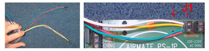
The red indicator (arrow) specifies the point ( 2 holes) where the wires need to be mounted to the Print Circuit Board with a tie-wrap.
