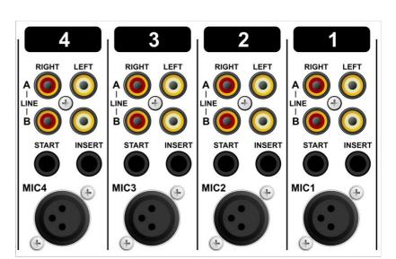
In order to use the **START** switch, it requires two pins in the <sup>1</sup>/<sub>4</sub>" stereo connector located on the back panel to be wired. The tip and ring are shorted when the ON switch or fader switch is activated. Once you have done this, you can start a turntable with the ON switch (if the START connector is wired on the back panel).
