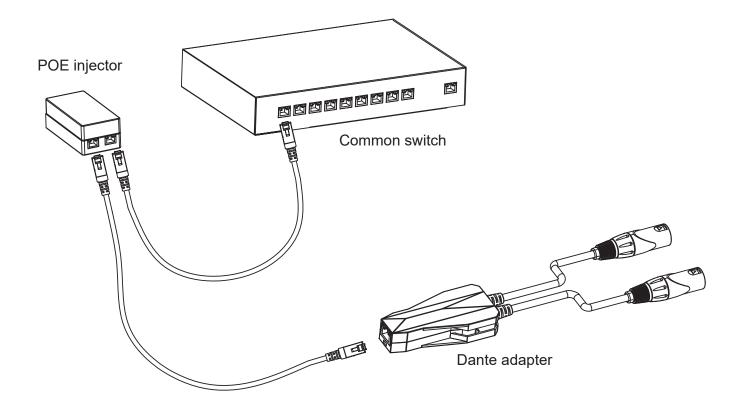
3. Ensure LED is solid on the RJ45 port of Dante adapter (Blinking yellow, solid Green)
