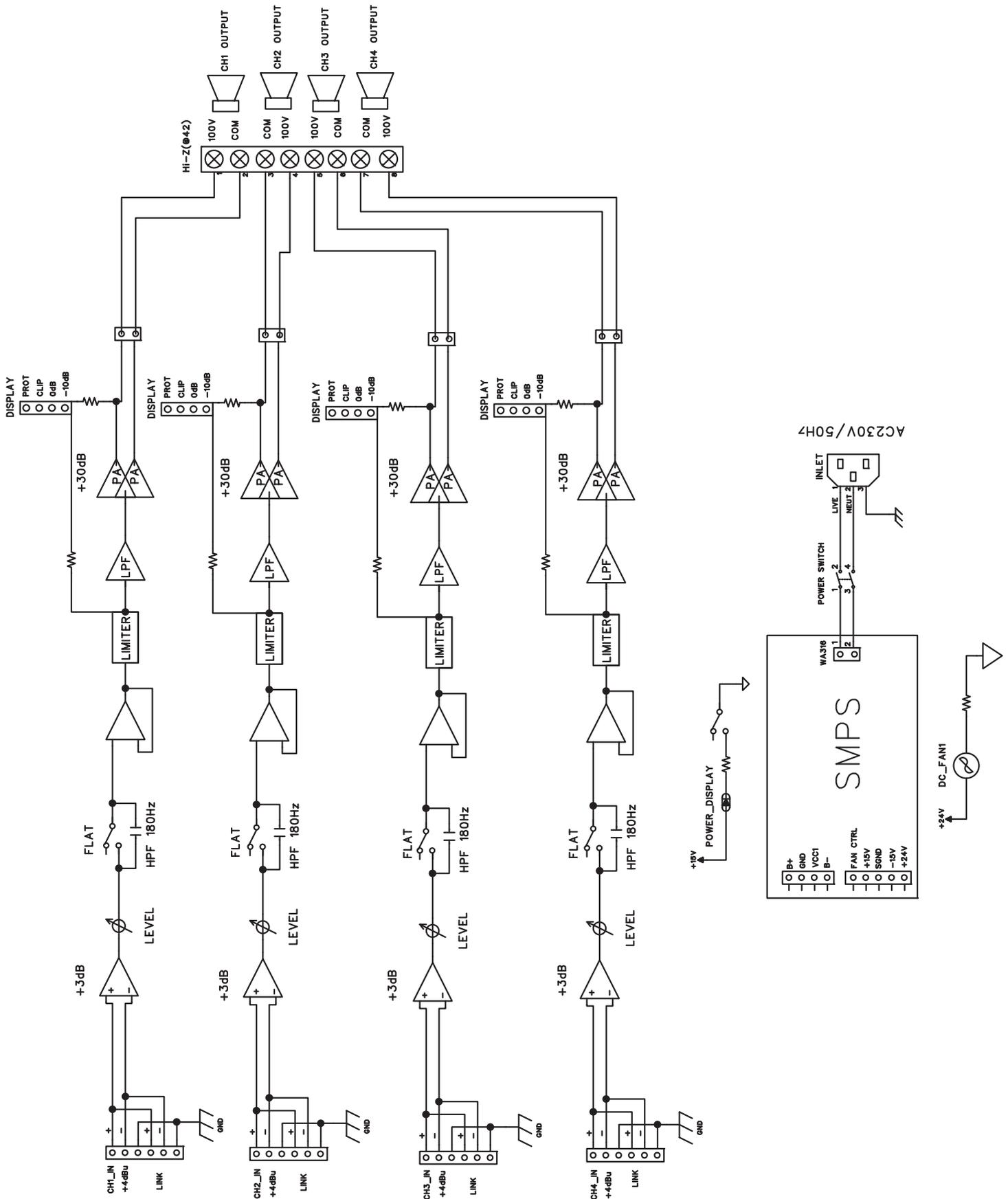
Note AMP480 is a mono-channel amplifier yet the synoptic is identical.
