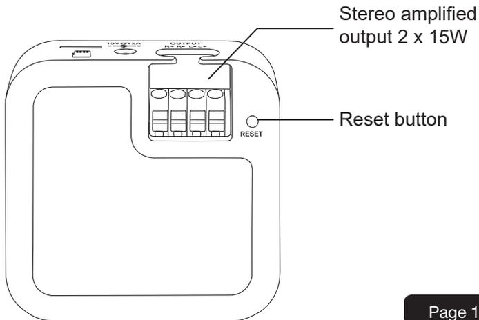
**Warning:** the impedance of the speakers connected to the WICASTamp must not be less than 8 Ohms
