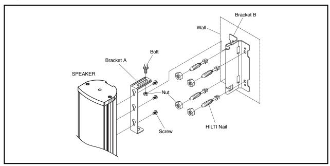
**WARNING:** under no circumstances should any loudspeaker be mounted or suspended in a public place unless the mounting method has been approved and certified by a qualified engineer. Failure to properly secure the system can result in damage to the unit or personal injury.
